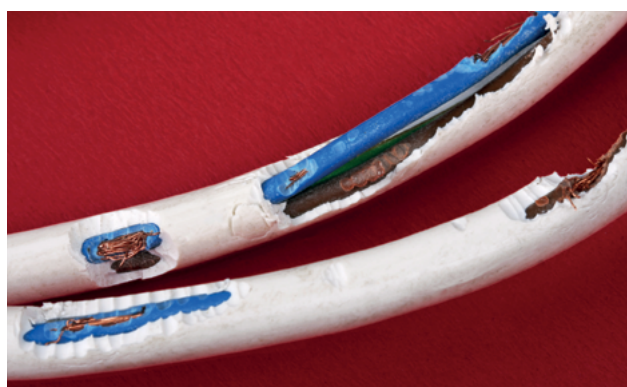
Fig. 11: Possible causes of series arc faults
